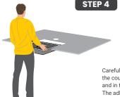
Carefully position the sink underneath the countertop, ensuring that it is level and in the correct position.
